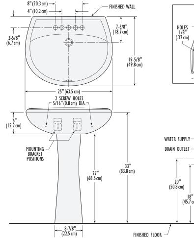
**IMPORTANT:** Dimensions of fixtures are nominal and may vary within the range of tolerance established by the standards ASME A112.19.2 / CSA B45.1 These measurements are subject to change or cancellation. No responsibility is assumed for use of superseded or voided pages.
