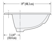
A.D.A. Lavatory Installation Requirements: Lavatories shall be mounted with rim/ counter surface no higher than 34 inches (86.4 cm) above finished floor. Provide a clearance range of 27 - 29 inches (68.6 - 73.7 cm) from the floor to the lavatory bottom or lavatory apron depending upon the type installed. For complete details on installation requirements, see A.D.A. Installation Handbook.
