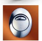
With the two-button Dual-Flush System control you can select a powerful, efficient 1.6 gpf/6.0 lpf flush for solid waste or a 1.1 gpf/4.0 lpf for liquid waste.
