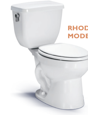
HURRICANE ADA HET MODEL 3140-3473 1.28 gpf/4.8 lpf 3" Flushing System ADA Compliant Flushes 1,000 grams of solids*
