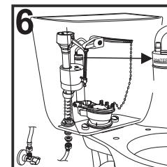
6.- Install the water supply line to the fill valve and turn on the water. Adjust water level to the water level mark inside the tank if necessary.
