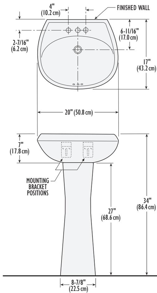
**IMPORTANT:** Dimensions of fixtures are nominal and may vary within the range of tolerance established by the standards ASME A112.19.2 / CSA B45.1. These measurements are subject to change or cancellation. No responsibility is assumed for use of superseded or voided pages.
